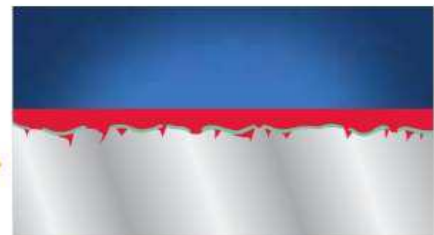
2. Enlarged section through the coated substrate shows Jotamastic penetrating down into the aged sound surface.
