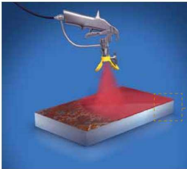
1. Jotamastic is applied to an aged coating in sound condition prepared to minimum St 2 (or even moist). Waterjetting prepared surfaces with early flash rust are acceptable. Good flow properties mean a smooth, consistent protective film. Low surface tension gives excellent wetting properties.
