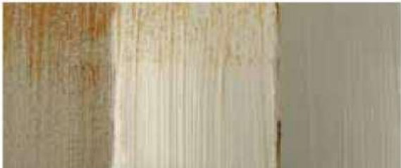
Typical brush application of traditional epoxy mastic coatings (left & centre) and Jotamastic Smart Pack (right) after continuous exposure in a salt water chamber. Rust penetration is apparent due to uneven film thickness being achieved after brush application – unlike Jotamastic Smart Pack with its superior flow characteristics achieving a consistent and correct film thickness.
